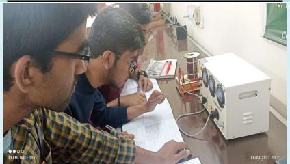
Study of tangent galvanometer: determination of reduction factor and horizontal component of Earth's magnetic field.
