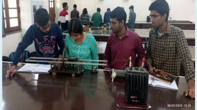
Study of Carrey Foster's bridge: determination of resistance per unit length of the bridge wire and of a given unknown resistance.
