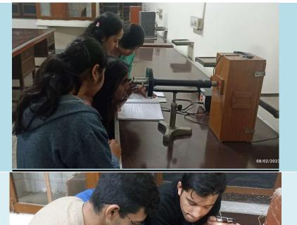
spectral lines of mercury (for violet, green, yellow-1 and yellow-2) using plane transmission grating.
