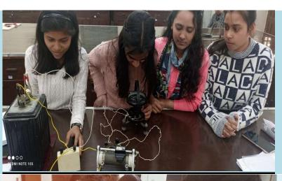
Determination of the wavelength of sodium light using Newton Rings' method.
