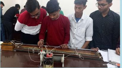
Determination of specific charge (charge to mass ratio; e/m) for electron.
